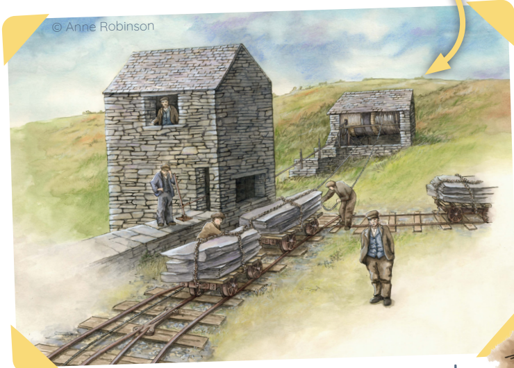
Trucks were attached to metal rope wound round a drum to go down the steep incline
